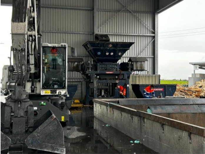
Electric excavator and shredder
